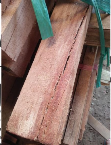
Gambar 5.12 Cacat Ring Shake
