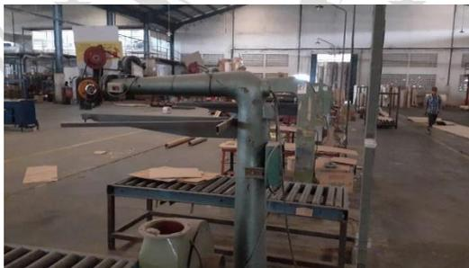
*Gambar 2. 8 Mesin Stitching*
