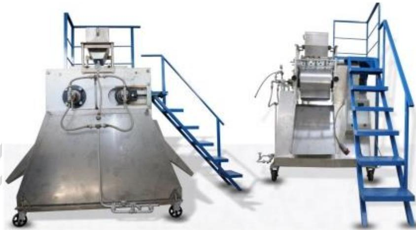
**Gambar 4.** Mesin *drum dryer* (Hidayat et al., 2021).
