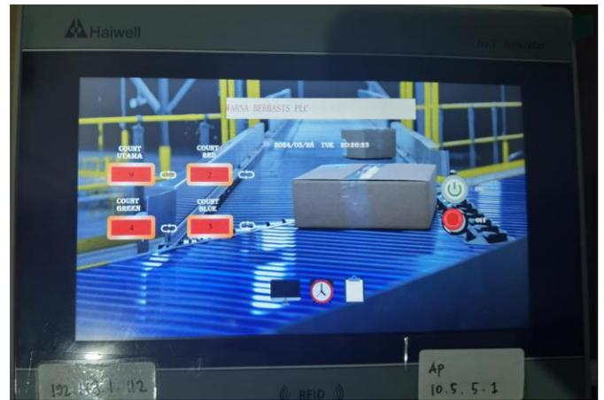
Gambar 5. Tampilan Counter Pada HMI
