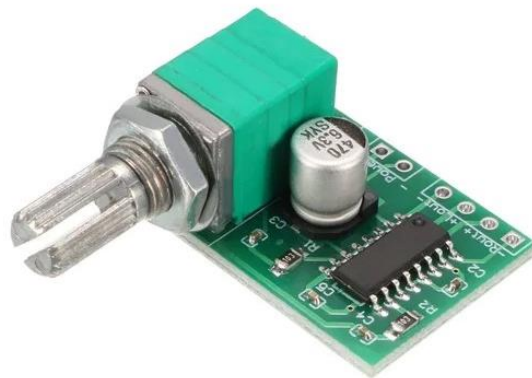
Gambar 2.8 Module amplifier PAM8403
