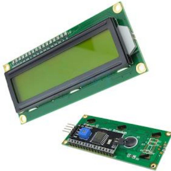
Gambar 2.5 LCD I2C 16x2
