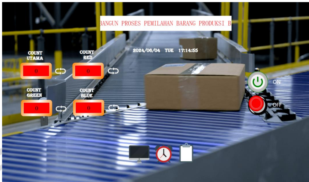
Gambar 1.4 Tampilan Main Display HMI
