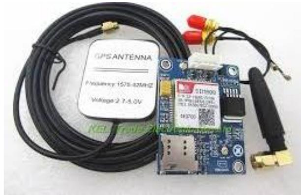
**Gambar 2.2** SIM808 GSM GPS Shield
