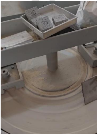
Pengujian Keausan paving block
