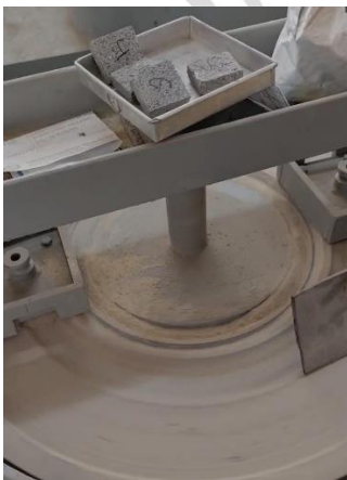
Pengujian Keausan Paving block
