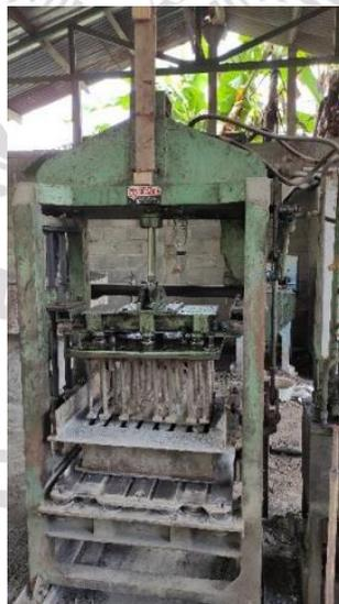
Gambar 2.11 Mesin *Hydraulic Pressure*
