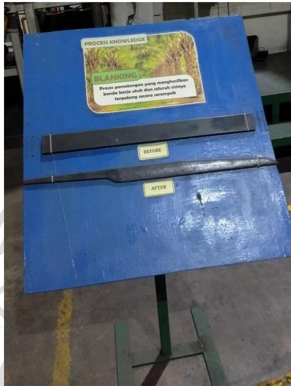
**Gambar 1. 5** Proses Knowledge Mesin Blanking
