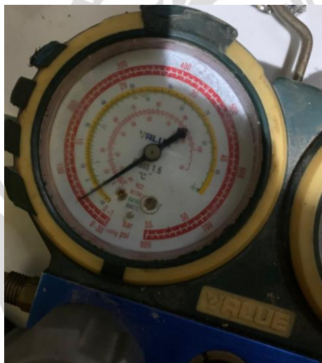
Lampiran 3. Tekanan sistem refrigrasi cold storage .
