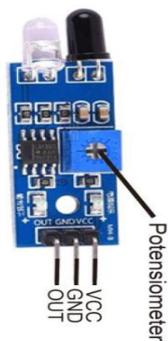
**Gambar 2.** Sensor Kecepatan IR Infrared Barrier Obstacle Avoidance
