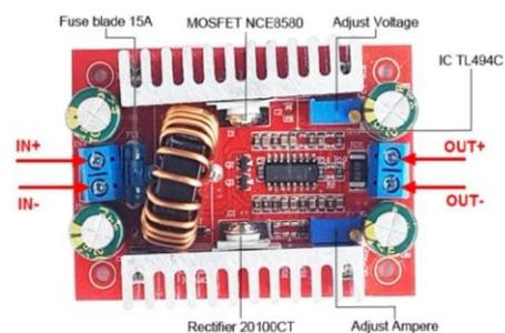
**Gambar 8.** DC-DC Step Up Converter 400W
