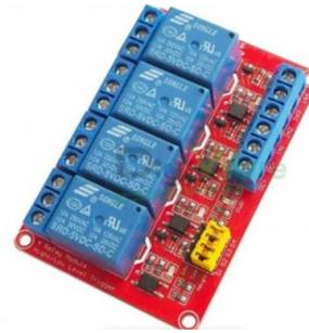
**Gambar 7.** Relay 4 Channel
