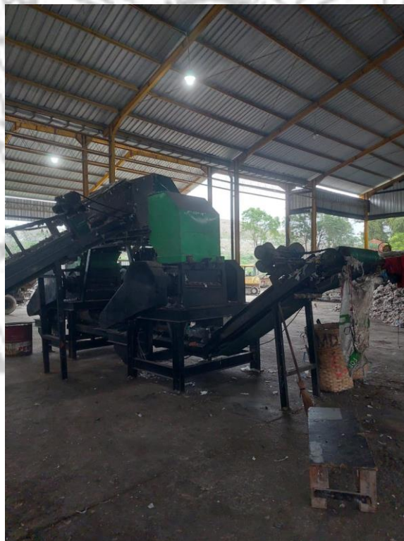
Lampiran 7 Mesin crusher
