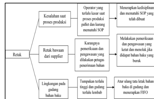
Figure 4. Tree Diagram of Causes of Wood Cracks
