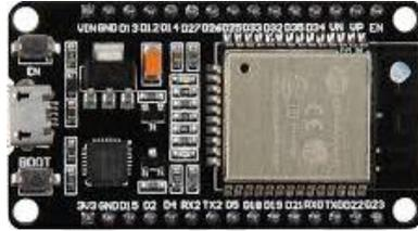
**Gambar 2.1** Microcontroller ESP32
