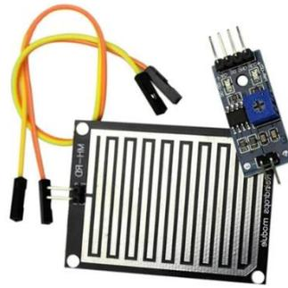
**Gambar 2.4** Raindrops Detection Module
