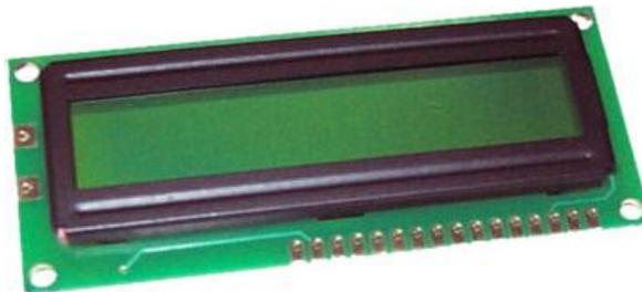
**Gambar 2.10.** *Liquid Cristal Display* (LCD) 2x16
