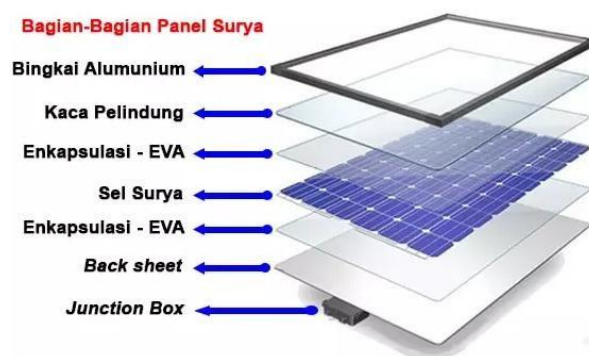
Gambar 2. 2 Bagian-bagian Panel Surya (sumber: https://zeusbattery.id/ )
