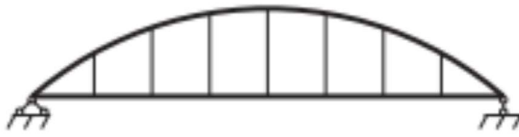
Gambar 2.2 Lantai Kendaraan Jenis Through Arch (Sumber: W.-F. Chen & Duan, 2014)
