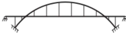
Gambar 2.3 Lantai Kendaraan Jenis Half-through Arch (Sumber: W.-F. Chen & Duan, 2014)
