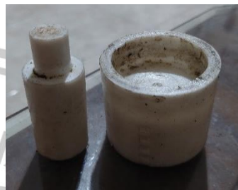
Teflon road sesudah di bubut, disesuaikan diameter inner dan outer bearing
