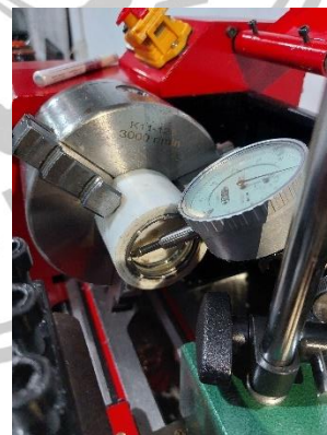
Pengujian kerataan outer bearing
