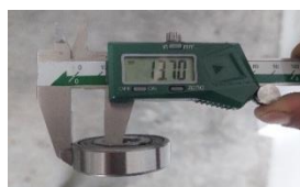
Pengukuran ketebalan bearing
