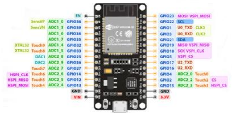
Figure 1. ESP32 Architecture and Pin Out
