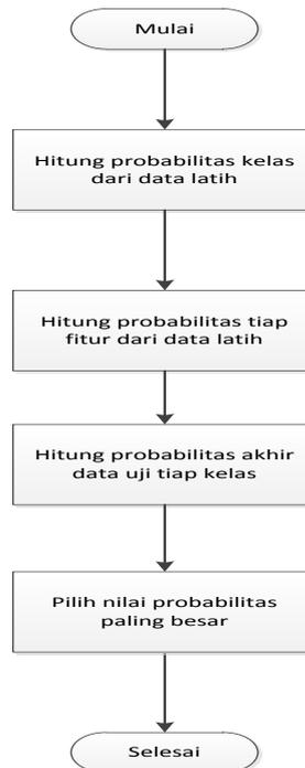
**Gambar 3.2** Flowchart sistem algoritma Naive Bayes
