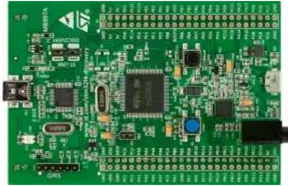
Gambar 2.15. ARM STM32F4 Discovery board ( www.st.com , 2015)
