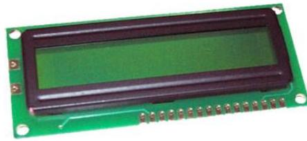
**Gambar 2.31** *Liquid Cristal Display (LCD) 2 × 16*
