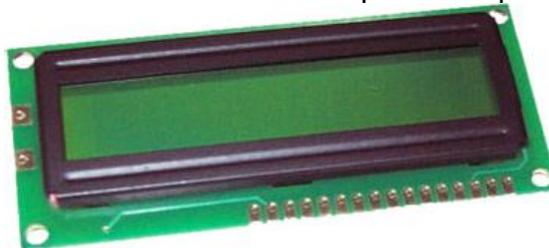
**Gambar 2.9.** *Liquid Cristal Display (LCD) 2x16*
