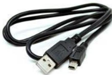
**Gambar 2.9** Kabel USB Board Nuvoton NUC 120
