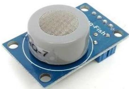
Gambar 2.4 Sensor gas MQ-7
