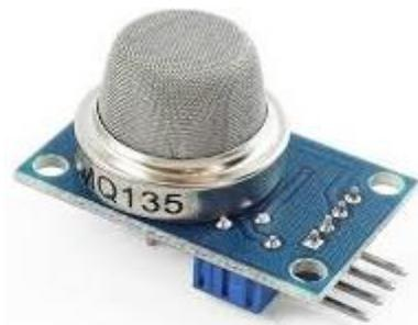
Gambar 2.6 Sensor gas MQ-135
