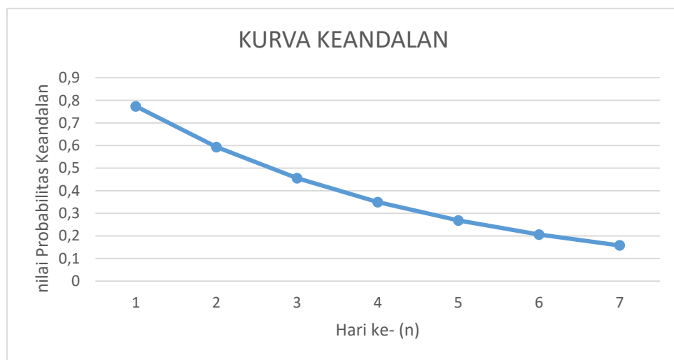
Gambar 5.1 Grafik Keandalan/Reliabilitas mesin Hanger Shot Blast
