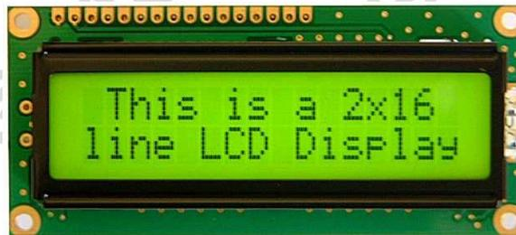
**Gambar 2.6** LCD (*Liquid Crystal Display*)
