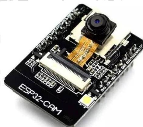
**Gambar 2. 6** Modul ESP32-CAM
