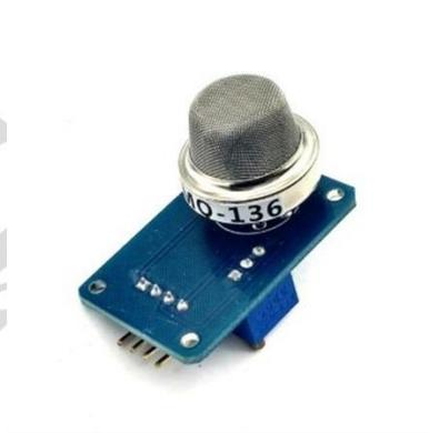
**Gambar 2. 8** Sensor gas MQ-136
