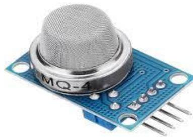
**Gambar 2. 23** Sensor gas MQ-4
