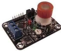
**Gambar 2. 19** Sensor gas MQ-3
