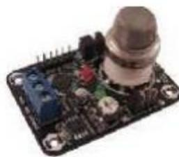
**Gambar 2. 7 Gambar Sensor gas MQ-135**
