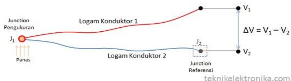
Gambar 2.3. Prinsip kerja termokopel
