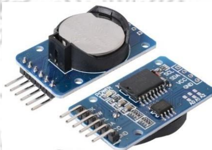
Gambar 2.19 Modul RTC DS3231
