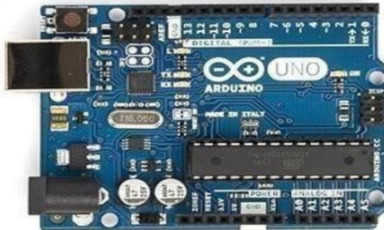
Gambar 2.5 Hardware Arduino Uno
