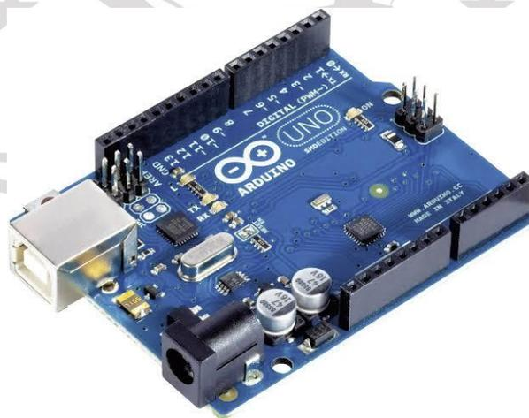
**Gambar 2. 14 Board Arduino Uno**
