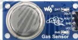
**Gambar 2.6.** Sensor Asap MQ2
