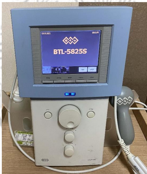
Gambar 2.7 Apparatus for laser therapy, electrotherapy and ultrasound therapy BTL 5825 SL (Sumber : Dok. Pribadi)
