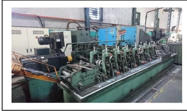
Gambar 2.4 Mesin *Forming line 1*
