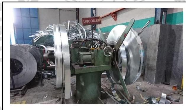
Gambar 2.2 Mesin *Uncoiler* line 1
