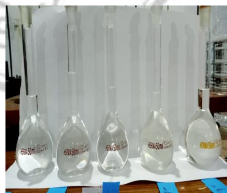
Gambar 6.5.5 Larutan standar quersetin 2,4,6,8,10 ppm
