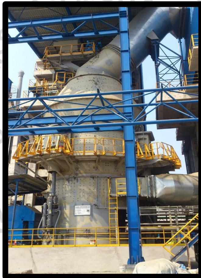
Gambar 2.1 Mesin *Vertical Roller Mill*
