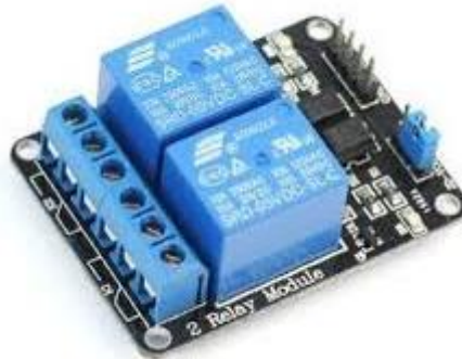
Gambar 2. 6 Transfer Switch Relay
