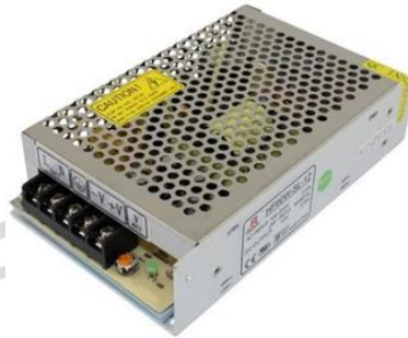
Gambar 1.12 Modul Power Supply Switching 12V 10A
