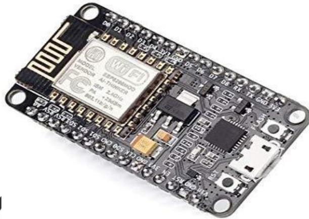
Gambar 2.2 Arduino NodeMCU esp8266
