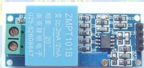
**Gambar 2.7** Sensor Tegangan ZMPT101B
