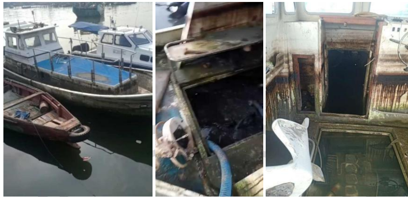
Picture6 Vessel Before Docking (Draining)
