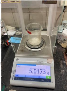
Gambar 2. 6 Proses penimbangan sampel pengujian Insoluble Matter
