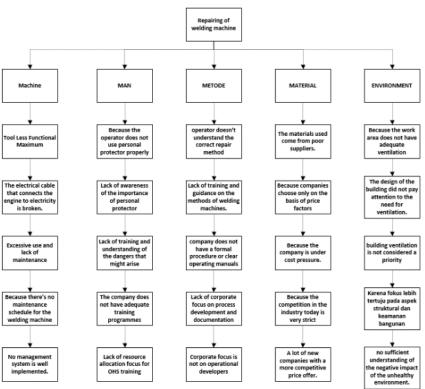
Figure 6 Rca operrating welding machine
