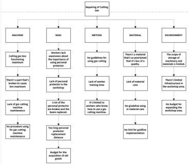
Figure 7 Rca operating cutting gas
