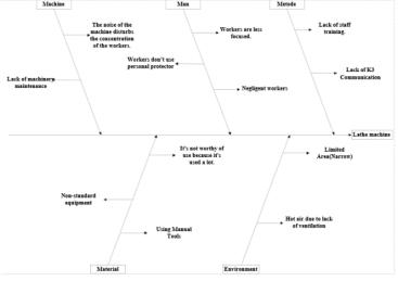
Figure 2 Fishbone repairing lathe machine
